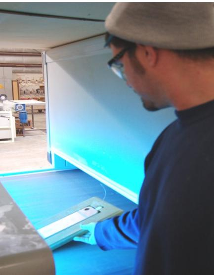
*An Omega Cabinetry operator sends an EIT Power MAP down the UV flat line.*
