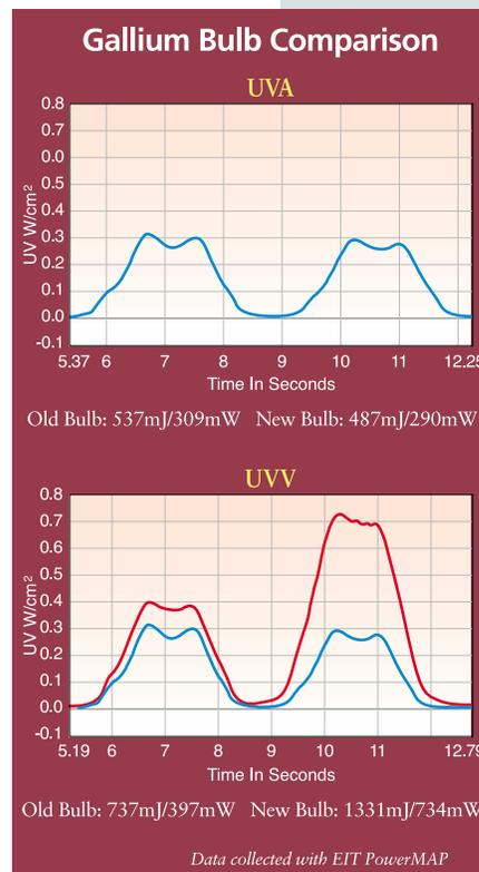
Figure 16: Looking at only the UVA, the old and new bulbs appear to be similar in output. There is quite a difference in the output of UVV with the new bulb significantly. It is important to sometimes measure more than a single UV bandwidth. (Information originally collected by Efsen Engineering).
