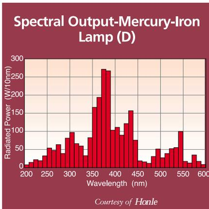
Figure 18: Typical Spectral output from a Mercury-Iron Lamp (Courtesy of Honle).
