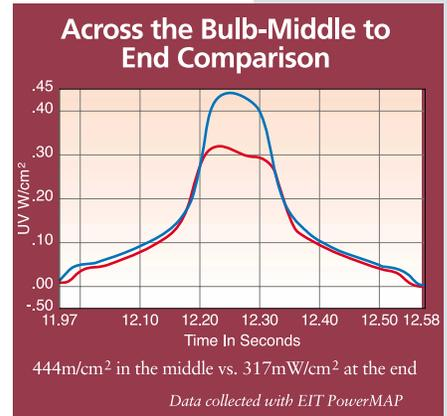
Figure 9: Comparison of measurements at the end of the bulb, versus near the middle. If the readings are lower in the middle than on the end, opposite of what is shown here, check the positioning of the bulb and look for sag.
