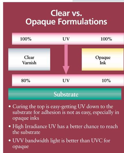
Figure 20: There are differences when curing clear and opaque coatings. Work with your suppliers to understand and establish the amount and type of UV needed for your coatings.
