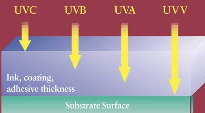
Figure 15: The longer wavelengths have a better chance for penetrating through coatings than the shorter wavelengths.
