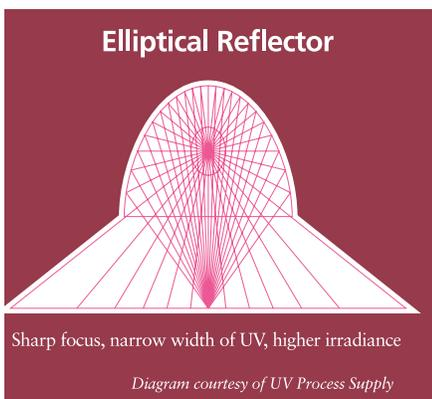
Figure 5: Typical light pattern from an Elliptical Reflector design.
