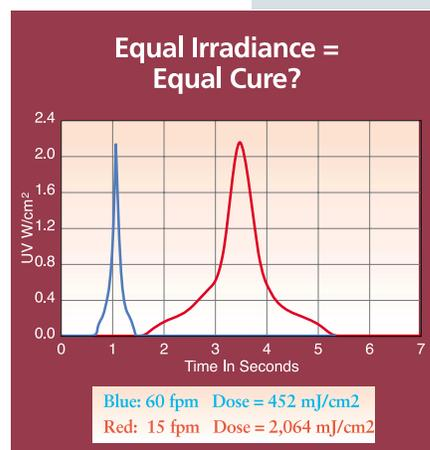
Figure 21: Equal numbers of Watts do not always lead to equal cure characteristics. It is important to establish and maintain energy density levels for your process.
