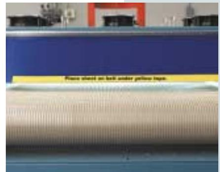
Figure 10: Yellow tape attached to the UV system to guide product placement on the UV conveyor (Photo courtesy of Avery Dennison).
