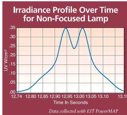
Figure 8: Typical light pattern from lamp that is out of focus. It is important to confirm if your process and equipment was designed to run out of focus or if the out of focus condition is a change due to a bulb sagging or lack of maintenance.
