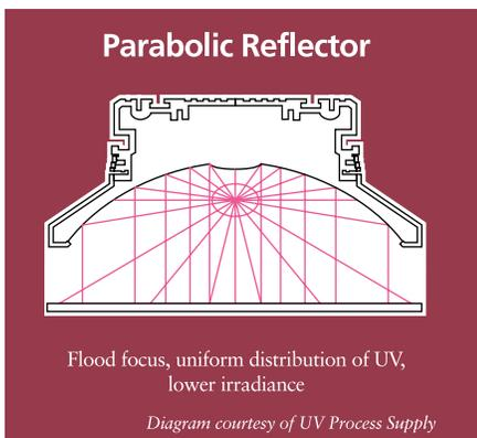
Figure 6: Typical light pattern from a Parabolic Reflector design.
