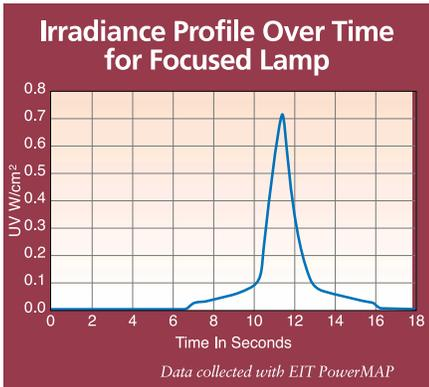
Figure 7: Clearly defined profile shape from a focused lamp, often produces higher irradiance values.
