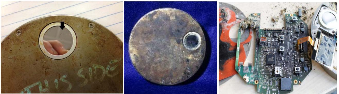
*Above Left & Center: Radiometers in need of better care Above Right: Radiometer that took a swim in coatings*
