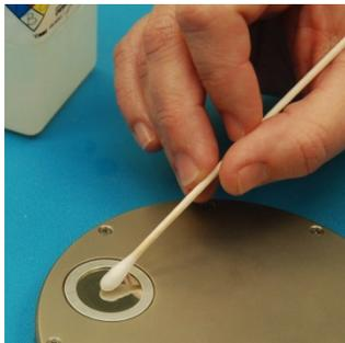
If using cotton **SWABS**, apply a liberal amount of isopropyl alcohol to the tip. Use sufficient alcohol to thoroughly wet the swab. Moving quickly (since the alcohol evaporates), use a back-and-forth motion while rotating the shaft of the swab between your fingers, clean the surface. Never reuse a swab. If more cleaning use another swab since used swabs will contaminate the surface. Use a clean dry swab to remove excess alcohol.
