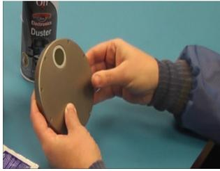
Visually **INSPECT** the optical surface for signs of contamination, residue, fingerprints and loose debris on or near the optical window.
