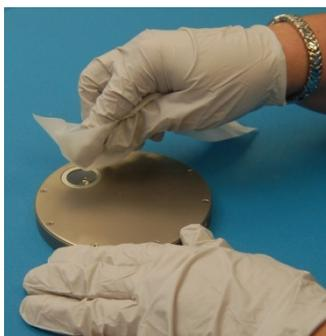
Gather some of the wipe between the thumb and forefinger for cleaning. Using the gathered material, **CLEAN** the surface using a firm but gentle motion. Re-gather the wipe material occasionally so that clean, wet portions of the wipe are used to clean the surface. Repeat this procedure until the surface is clean. Always **DISPOSE** of the wipe and packaging safely, according to the instructions on the packaging.
