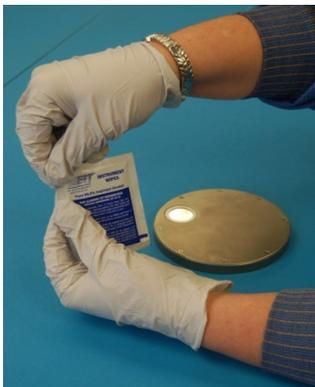
If using prepackaged EIT chemical **WIPES**, put on clean, disposable rubber gloves. Handle gloves from the ends. Never touch the fingers of the glove with bare hands. Gloves protect the skin and prevent oils from the skin contaminating wipe. Tear open the foil packaging, remove the wipe and unfold it gently.
