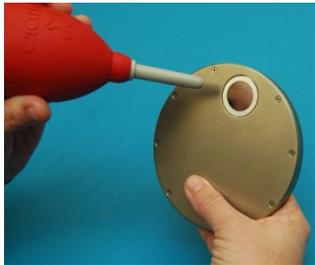
**BLOW** any loose particulates free by holding the device vertically. Using an air bulb, clean, dry compressed air, or residue-free aerosol chemical de-duster remove loose dirt. When using de-duster, position the nozzle 10"-12" from the optical surface so that the de-duster doesn't build up on the window surface. Using the rapid moving air, not the chemical itself to blow the surface clean.
