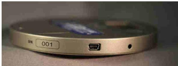
Above: Side view of instrument showing Serial Number, USB port and Alarm
